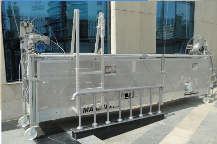
1,5 m mesh cladded Light Weight Cage for permanent installation with CX500 hoist, Sky Lock, wire winder and access ladder
