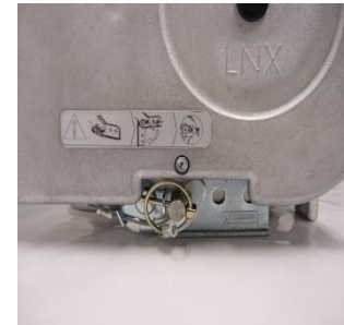
Retractable stirrup strap Closed position:
